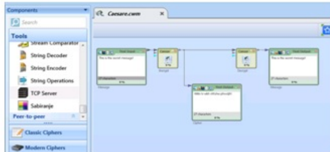
Figure 3. Using Caesar Cipher in Cryptool
